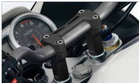
RISERS FOR OVERSIZE HANDLEBARS - BLACK Offered for use with Tiger oversize handlebars.
