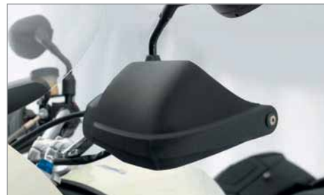
HAND GUARDS Durable molded nylon hand guards, offer substantial protection against wind and debris.
