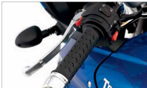
HEATED GRIP KIT Twin position heated grip kit, features internal wiring for neat installation and cockpit mounted switch.
