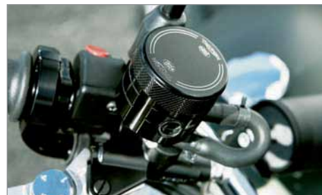
ANODIZED BRAKE RESERVOIR - FRONT Features sight glass and knurled lid, laser etched with Triumph logo.
